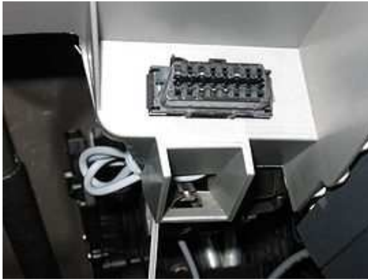
Fig. 3.2: Female 16-pin (2x8) J1962 connector
