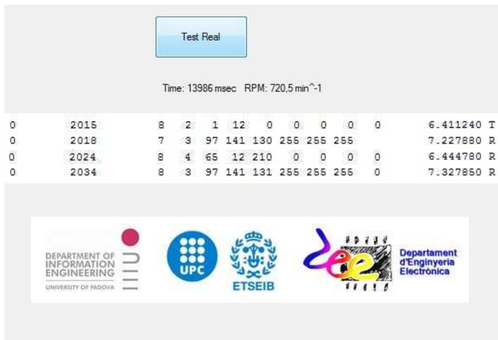
Fig. 6.4: CanKing Output Window and application screen for PID 0x0C
