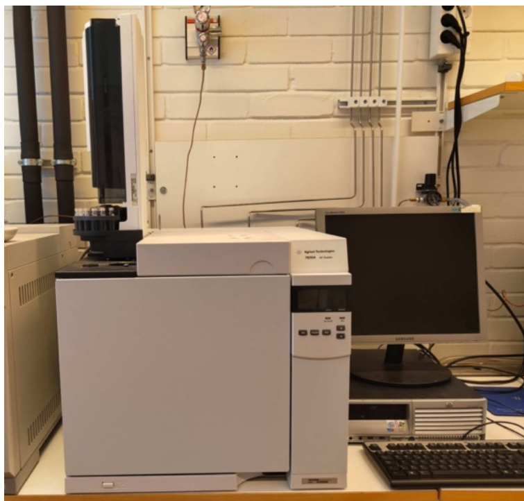
Figure 4.3 – Agilent 6890 N GC equipped a HP-5 MS capillary column and MS detector.
