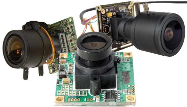
Figure 84: Examples of optoelectronic devices. Notice the mismatch between the sizes of the optical and electronic parts.
