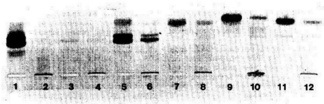
Figure 1.3: The SDS-PAGE of dairy proteins subjected to transglutaminase activity. Lanes 1 = whole casein, 3 = \alpha -casein, 5 = NDM, 7 = whey powder, 9 = \alpha -lactalbumin, 11 = \beta -lactoglobulin. Lanes 2, 4, 6, 8, 10, 12 are the respective substrates after reaction with transglutaminase.
