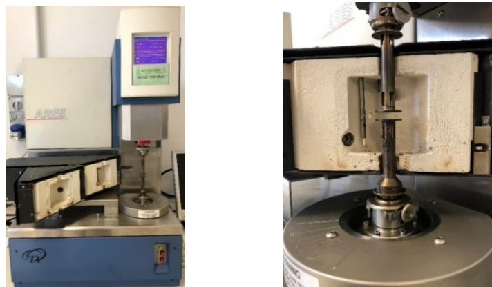
Figure 4-10 Rotational rheometer and cone-plate measuring system.
