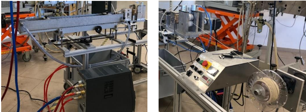
Figure 4-6 Cooling bath in the left and the pull system in the right.
