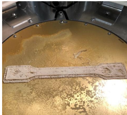
Figure 8-24 Failed printed due to the problem at the feeding system, gave from the contamination.
