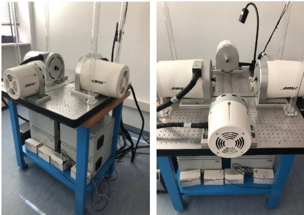
Figura 3.1 Sistema Bose® ElectroForce Planar Biaxial TestBench.
