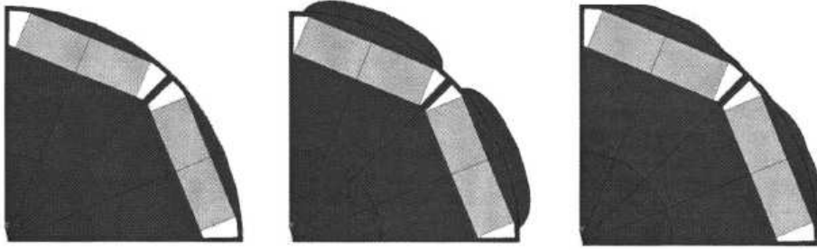
Figure 4.3: Different round shape design: from the left, conventional, sinusoidal, semi-block shape. [21]
