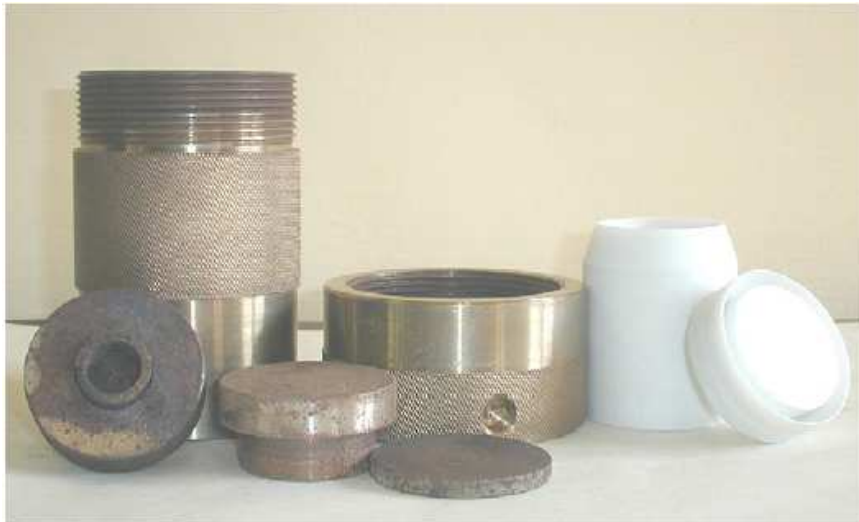
Figure 8-3 Example of autoclave used for hydrothermal treatment (34).
