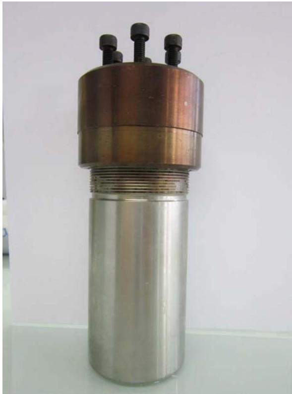
Figure 9-3 Autoclave used for the hydrothermal process.
