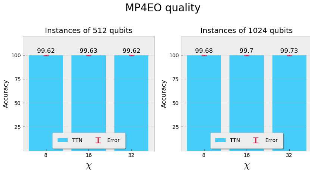
Figure 3.11: Mission accuracy for system with 512 and 1024 qubits, applying the TTN optimization algorithm, In the x-axis there are the bond dimension for the TTN optimizer, in the y-axis there is the mean accuracy of the missions, computed over different instances, with their error. The TTN algorithm shows a stable quality of the output even with the increasing of the system size.
