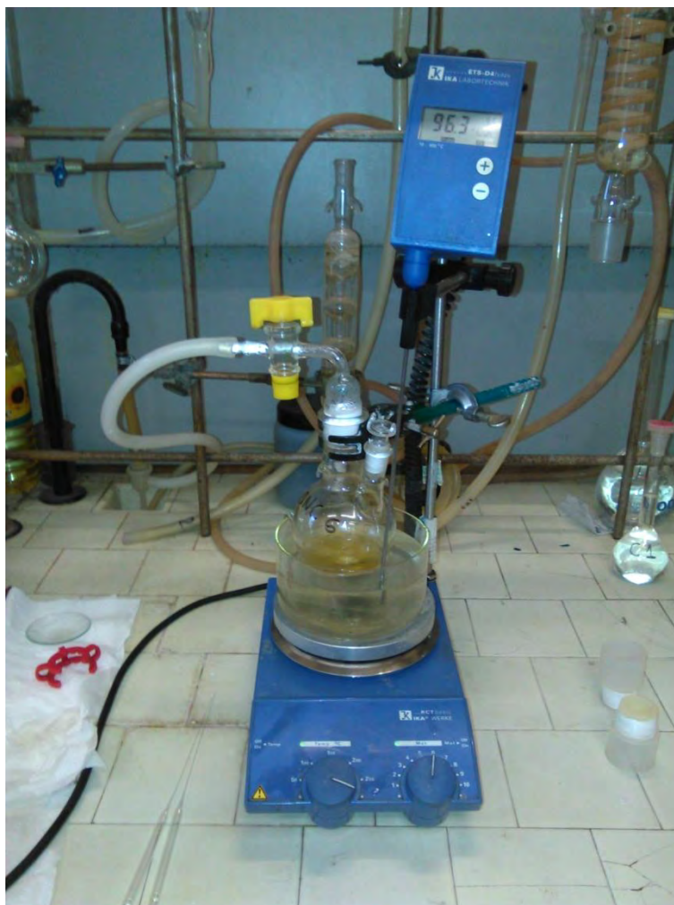
Figure 3.16 Evaporation of the solution thanks to the water pump during preparation for ICP analysis.
