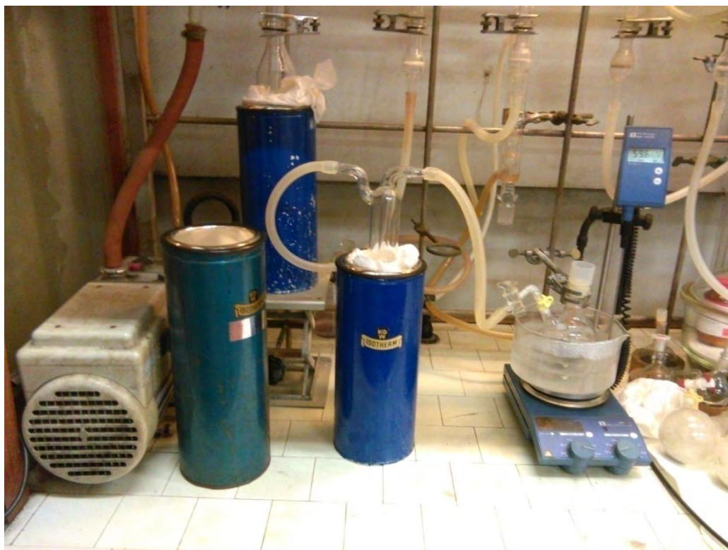
Figure 3.9 Vacuum drying of leachate sample.
