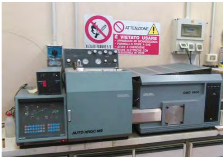
Figure 3.26 Carlo Erba GC-MS device.
