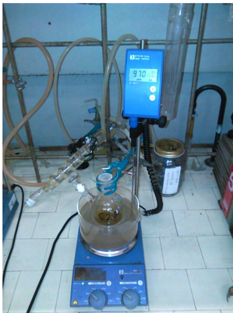
Figure 3.15 Leachate sample heated to 95°C ± 5°C and refluxed during preparation for ICP analysis.
