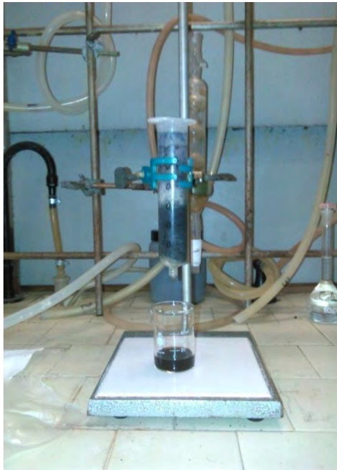
Figure 3.35 Leachate filtration by activated carbon.
