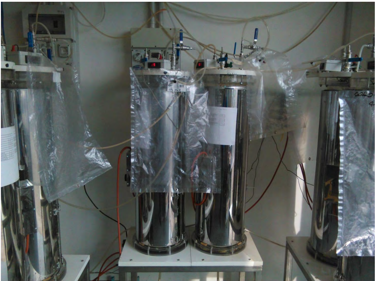
Figure 3.2 The six columns that simulate the landfill.
