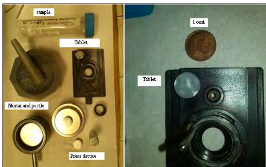
Figure 3.11 Instruments for the preparation of the tablet for the FT-IR analysis.
