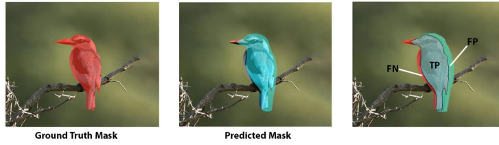
Figure 7.1: Graphical representation of IoU metric, from [9].
