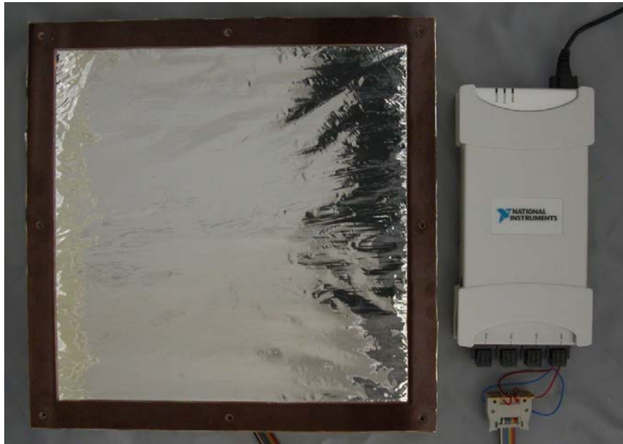
Figure 46 – On the left is represented the calorimetric system covered by the aluminized mylar foil. On the right is represented NI ENET-9219 data logger with relative connections.
