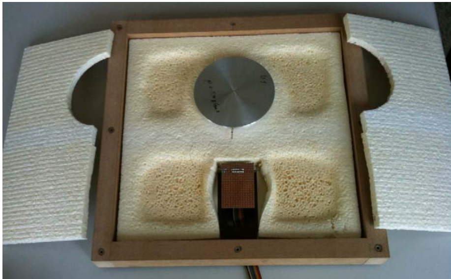
Figure 69 – Expanded Polystyrene melting after several passages under the electron beam. The consequences of the radiation can be seen in the yellow color of EPS and in the four melted zones around the aluminum calorimeter.
