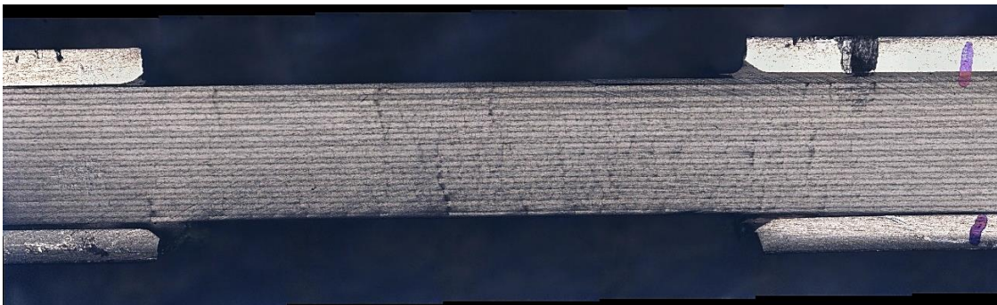
Figure 5.26: Cracks at 10000 cycles for "B23" sample at a lower magnification
