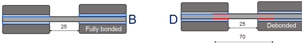
Figure 3.14: Final design and dimensions of B and D type specimens. Dimensions of tabs and coupon are not drawn to scale [30]
