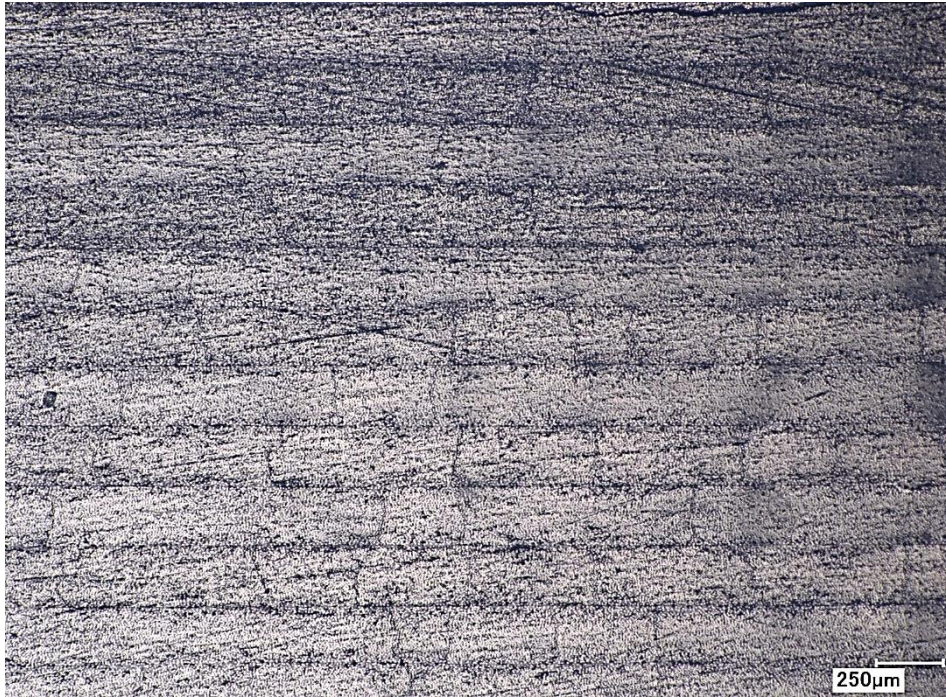
Figure 5.25: Cracks at 10000 cycles for "B23" sample
