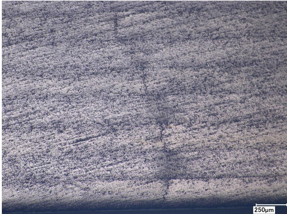
Figure 5.24: Cracks at 7000 cycles for “B23” sample
