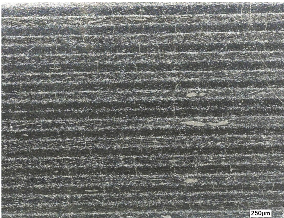
Figure 5.30: Cracks at 13000 cycles for "D16" sample at a lower magnification
