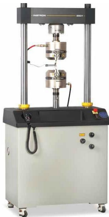
Figure 4.1: an Instron 8801 (100kN) servohydraulic fatigue testing system
