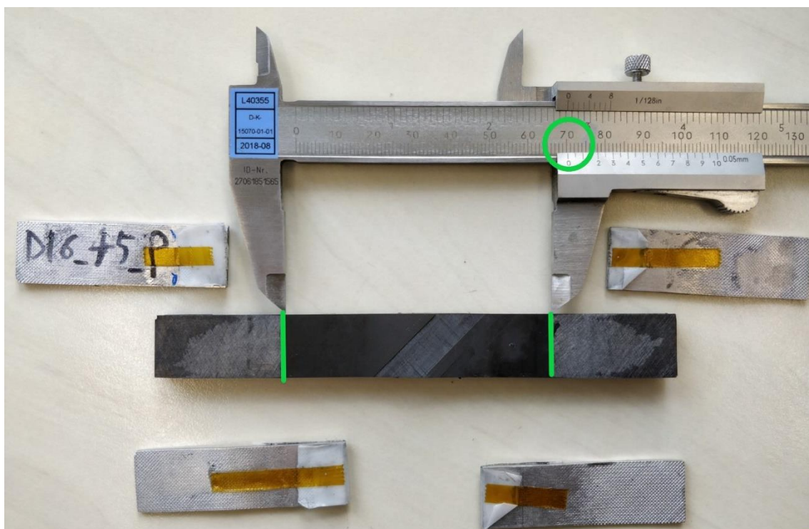
Figure 5.36: Tabs debonding surface after failure of "D16" specimen
