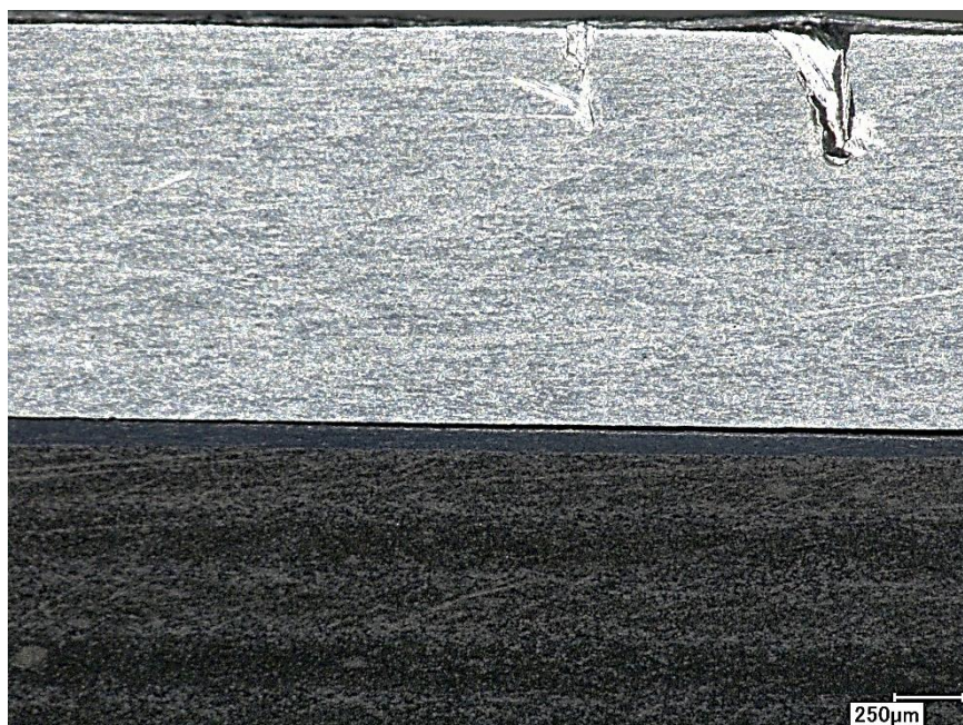
Figure 5.33: Tabs debonding at 3000 cycles for "B23"
