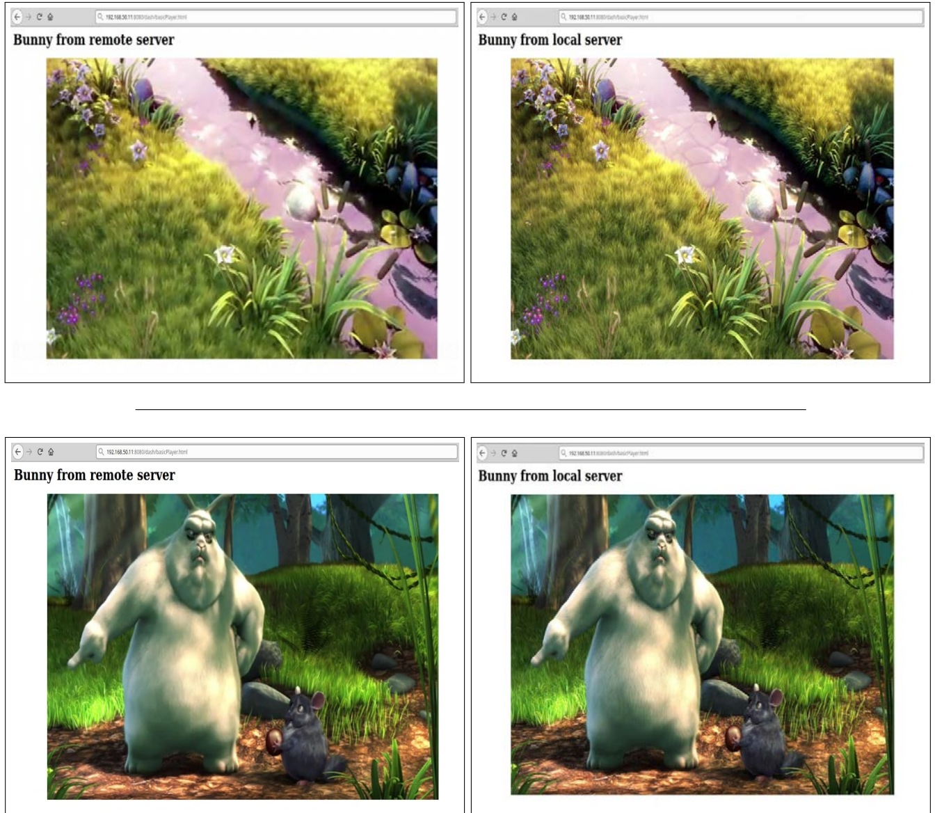
Figure 6.3: Comparison of two frames taken from the DASH stream at different qualities. The frames on the left belong to the stream from the remote server, the frames on the right to the stream from the local server. The remote stream reaches a top bitrate of 0.88 Mbps, whereas the local stream a top bitrate of 3.85 Mbps.
