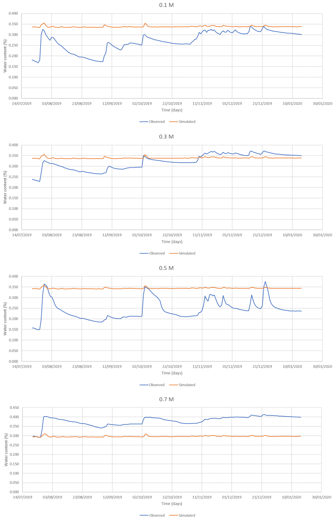
Figure 9. Water content dynamics of the third borehole
