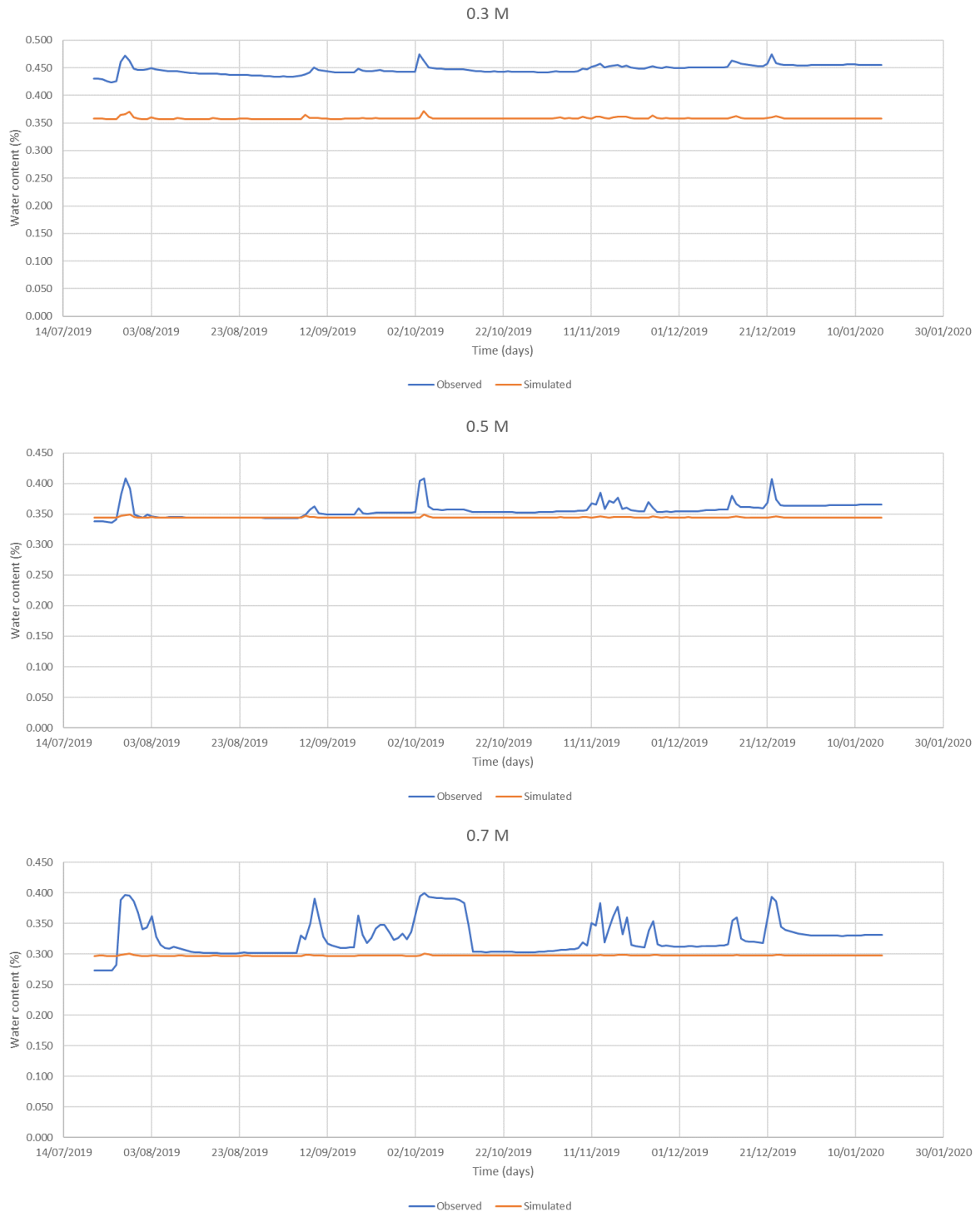
Figure 7. Water content dynamics of the first borehole
