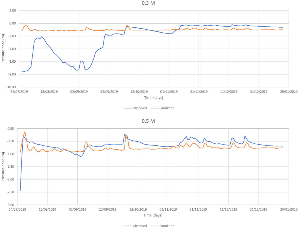
Figure 14. Water pressure head dynamic in the third borehole
