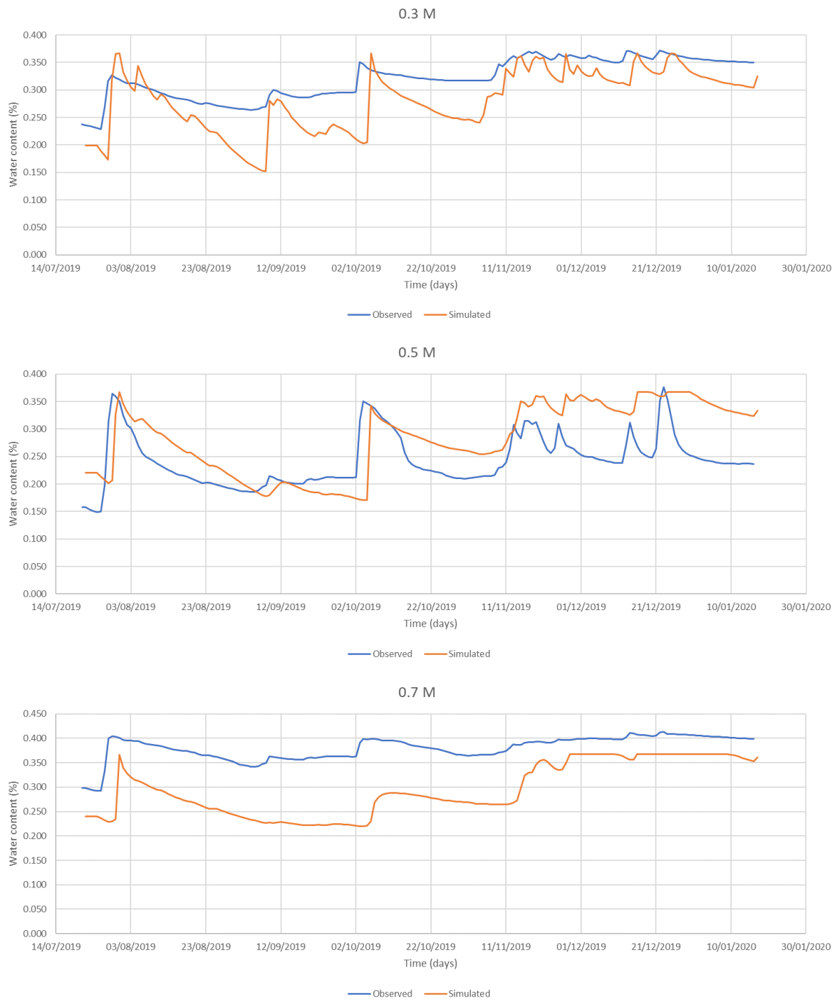
Figure 24. Water content dynamics of the third borehole after calibration
