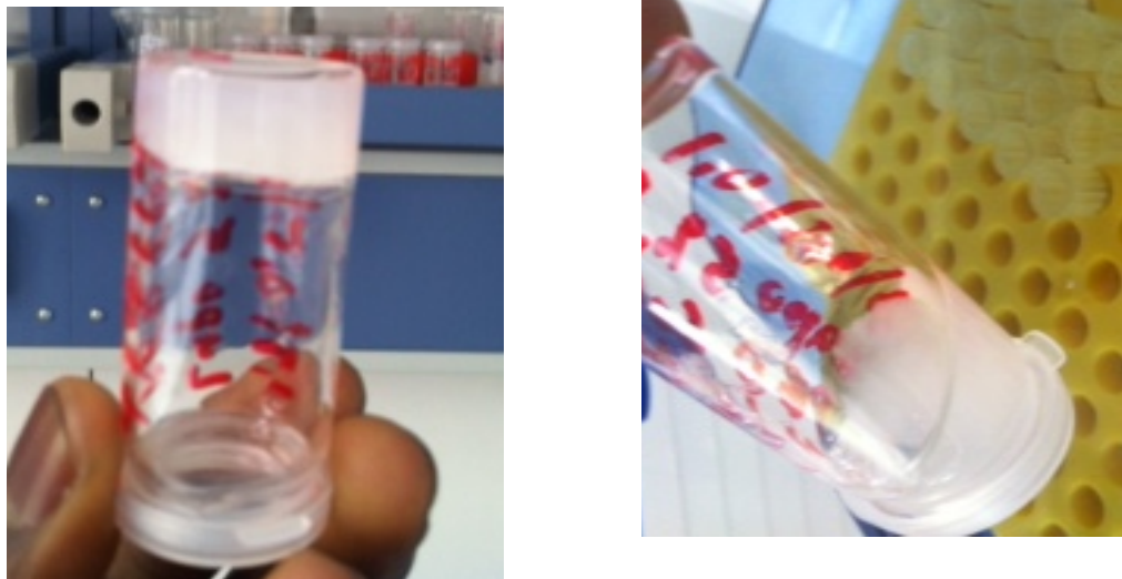
Figure 2.3. Samples of solid and sol gel that were formed upon inverting the vials.
