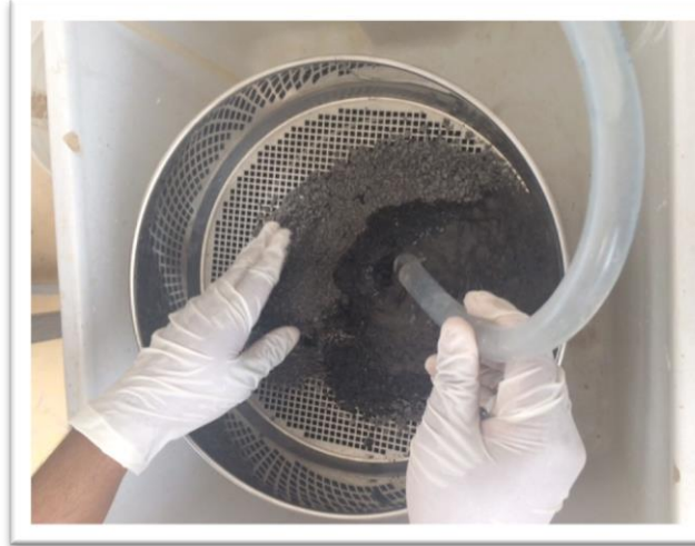
Figure 3: washing the material with water
