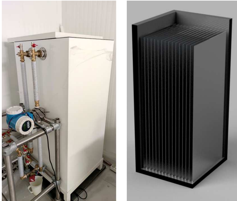
Figure 2.2: LTES Tank inside the climatic room, CAD model to illustrate the insides of the tank with the roll-bonds
