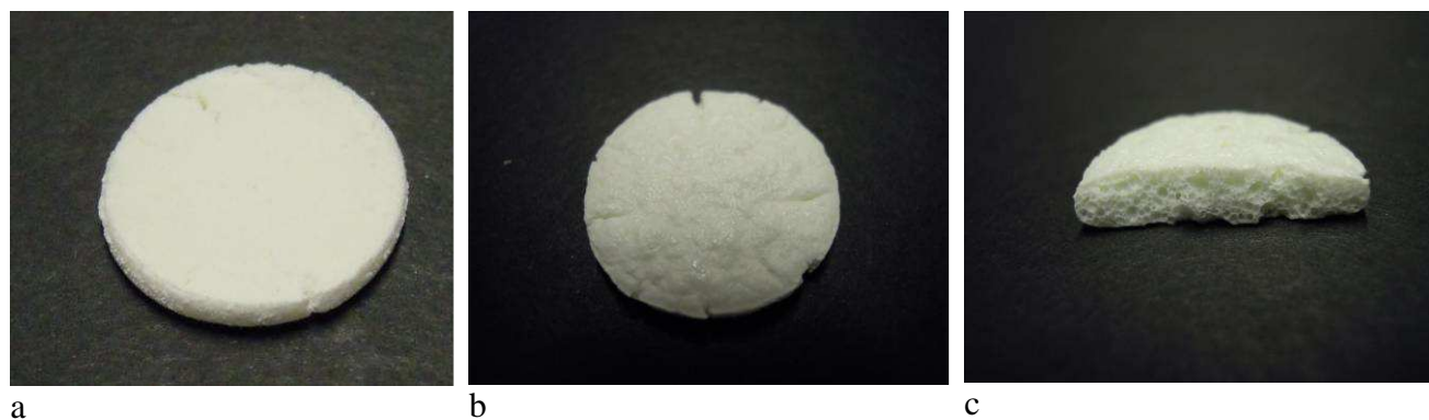
Figura 11.3. Trattamento 10°C/min. [a] TT5b (miscela base pura); [b] TT6b (90% miscela base, 10% soda-lime); [c] TT7b (80% miscela base, 20% soda-lime).
