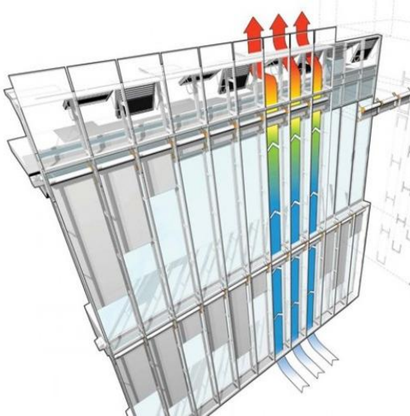
Figure 1.13: Representation of the natural raising of the air heated by the sun inside the DSF cavity.
