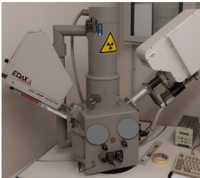
Figure 3.9: Leica Cambridge LEO 440 scanning electron microscope.
