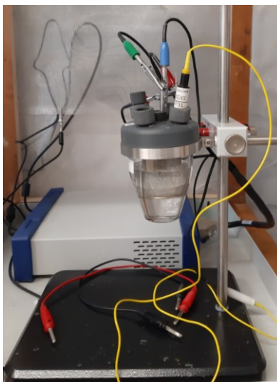
Figure 3.8: Traditional three-electrode implant; Platinum net as counter-electrode, sample as working electrode, saturated calomel electrode (SCE) as the reference electrode.
