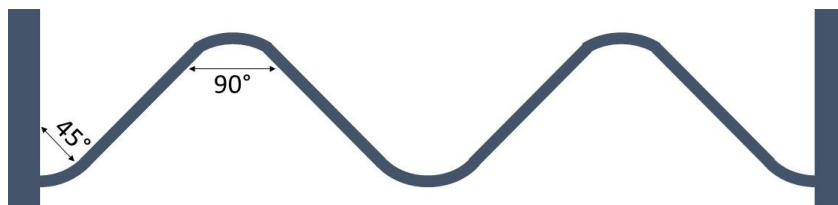
Figure A.8: Qualitative representation of the shape of the microchannels when two 45^\circ and three 90^\circ elbows are added.
