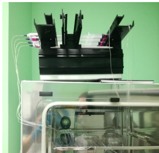
Figure 2.10: Experimental configuration during a biological experiment, where two \mu BRs, placed in the incubator, are connected to the syringe pump.
