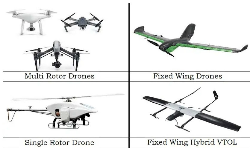
Figure 1.1: Small UAVs classification based on the propulsion system.
