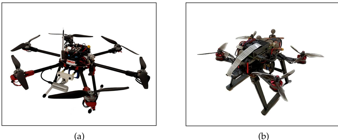
Figure 4.1: The two star-shaped multi-rotor platforms employed for the experiments, the hexarotor HR01 and the quadrotor QR01.
