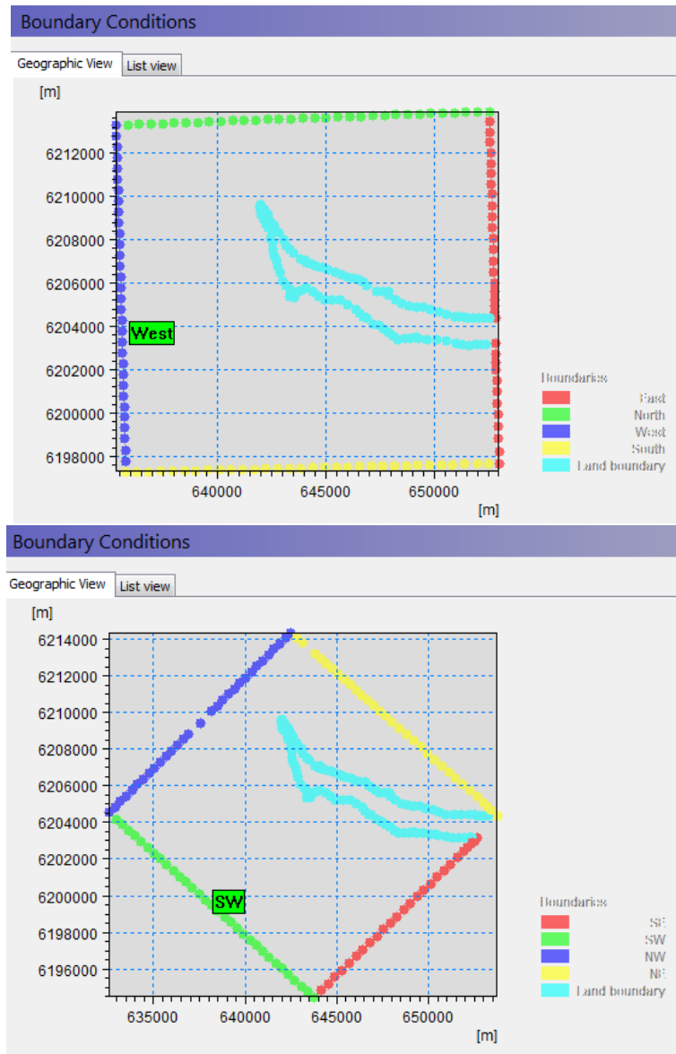
Figure 6.4: Representation of the boundary conditions for the principal directions (N, E, S, W), on the left, and the diagonal directions (NE, SE, SW, NW), on the right, as they appear in the program.
