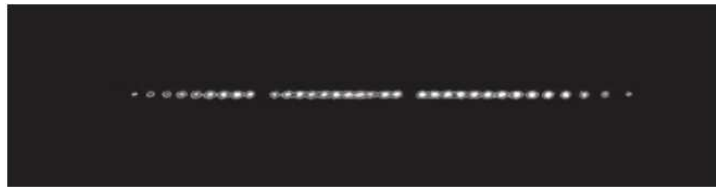
Figure 2.7: Image of fluorescence from about 40 trapped mercury ( ^{199}\text{Hg}^+ ) atomic ions. The ions are spaced by approximately 15 micrometers, and the two apparent gaps are different isotopes of mercury which do not respond to the probe laser. Reprinted courtesy of D. Wineland, at NIST.
