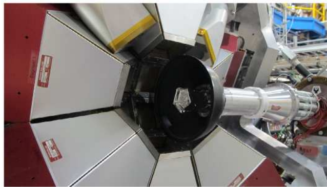
Figure 4.5: SCEPTAR and BGO (red and silver) around the HPGe [Garnsworthy et al., 2019].
