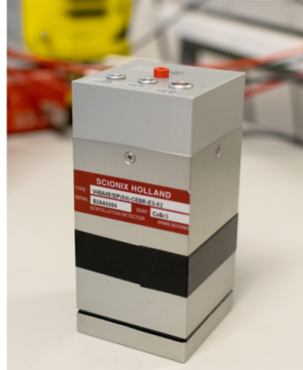
Figure 2.2: The scintillation detector. Figure provided by Oleksii Poleshchuk.
