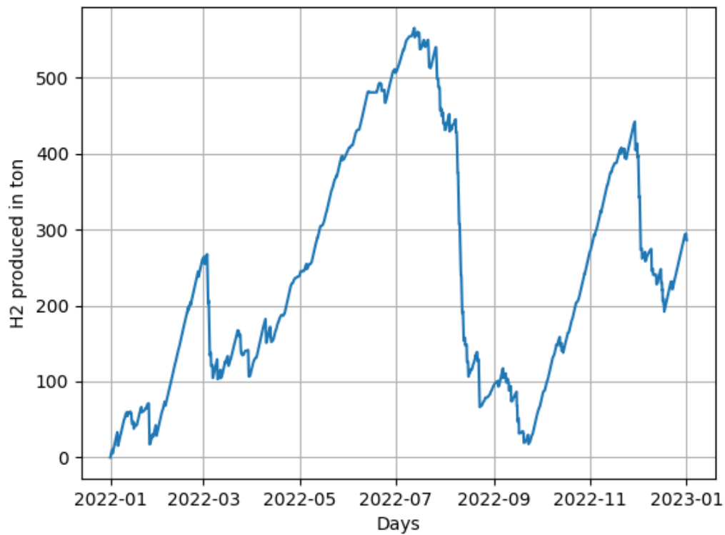
Figure 7.13: Cumulative difference of H_2 production and consumption for unit 1 with PEM power of 21.875 MW
