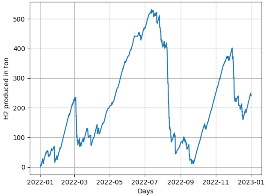
Figure 7.14: Cumulative difference of H_2 production and consumption for unit 1 with SOC power of 13.4 MW
