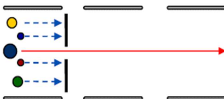
Figure 13, Schematic representation of the triple quadrupole analyzer in Q1MI configuration.
