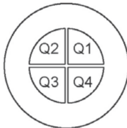
Figure 5.2: Scheme of the QPD sensor
