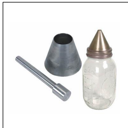
Figure 12 : (Pycnometer) Water Absorption and Specific Gravity Apparatus
