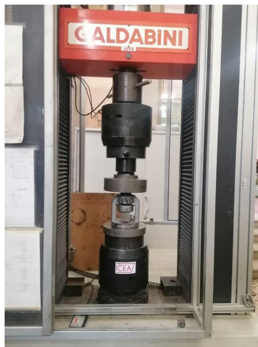
Figure 16: Compressive Strength Test Machine Used In Laboratory.
