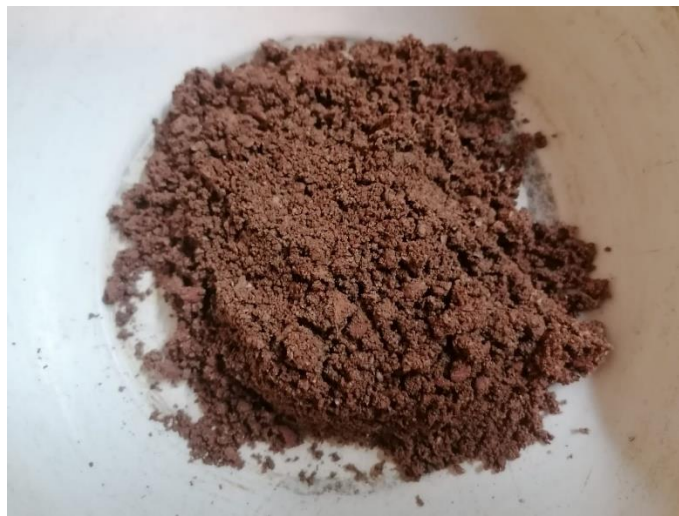
Figure 7 : Brick powder used in the laboratory.
