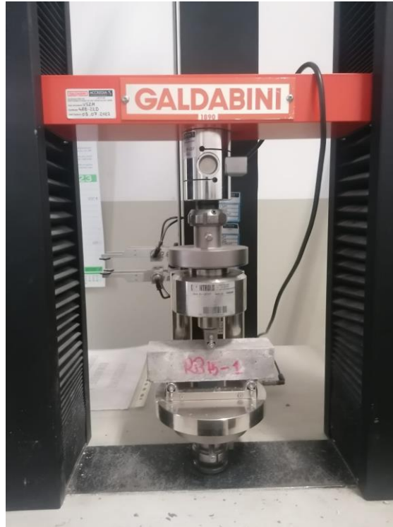
Figure 15 : The Flexural Strength Testing Machine Used In Laboratory.
