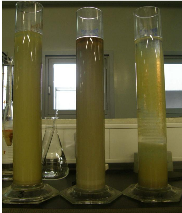
Figure 3.4 – Grain size analysis by sedimentation
