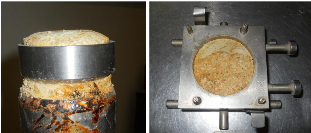
Figure 3.5 – Details of direct shear test: a) Specimen preparation; b) Sample positioned inside the shear box.
