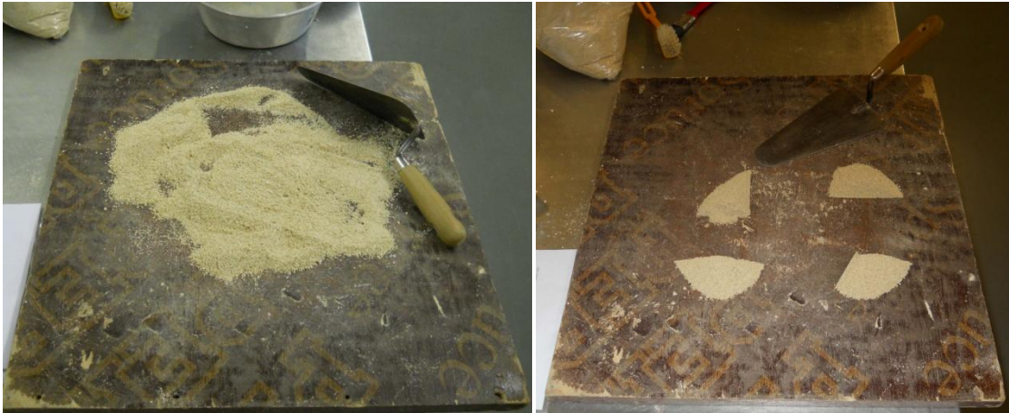
Figure 3.2 – Preparation of 25g soil to be placed into the flask
