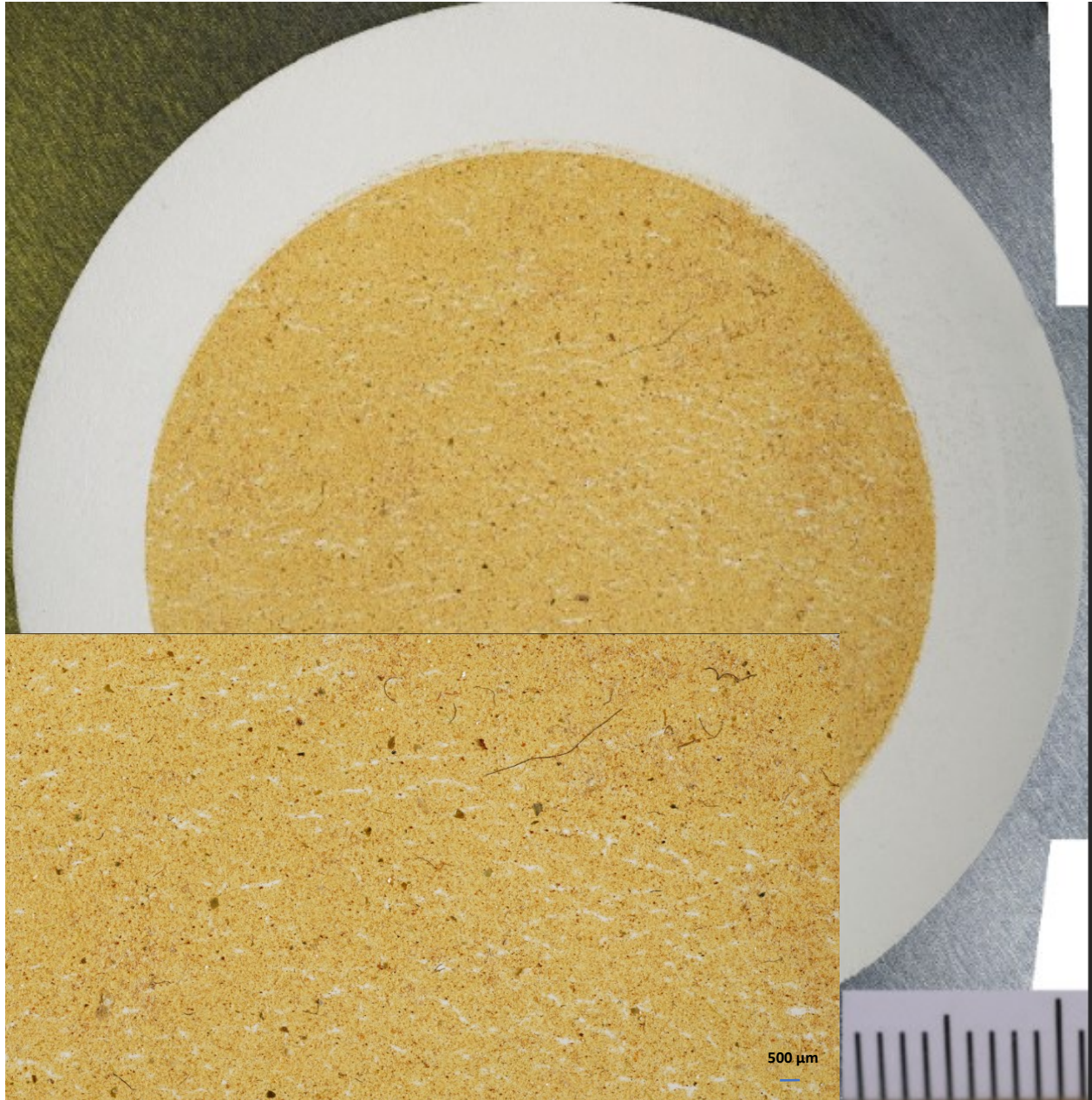
App.1: Filter from the water sample showing the distribution of different sizes for the PES fibers
