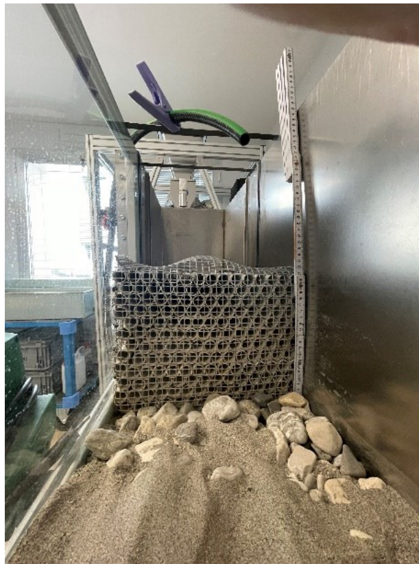
Figure 5: Pipes barrier with gravels downstream the barrier
