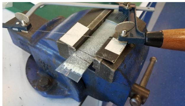
Figure 2.20: Specimen cutting using an hand saw.
