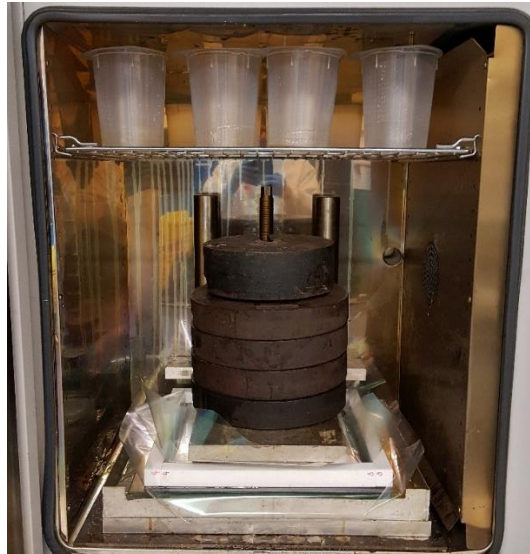
Figure 2.6: Composite inside the oven during the curing cycle with the weights on top.
