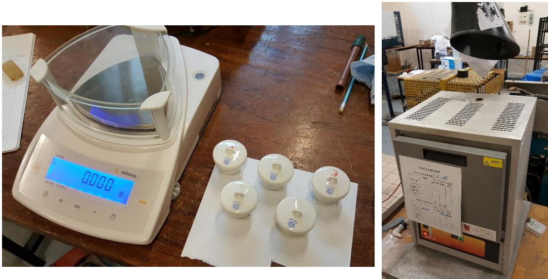
Figure 2.8: On the right can be seen the cups with the lid, inside them there are the samples and can be also seen the balance used. On the left there is the the furnace with the suction system for the fumes.
