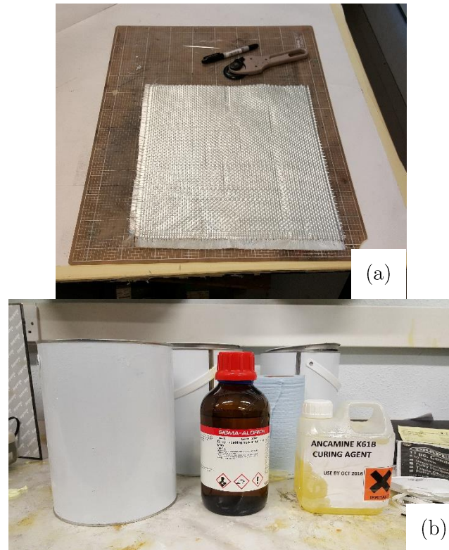
Figure 2.1: (a) the fabric is first cut from the roll using a pizza-cutter, (b) the three components of the resin are here depicted.
