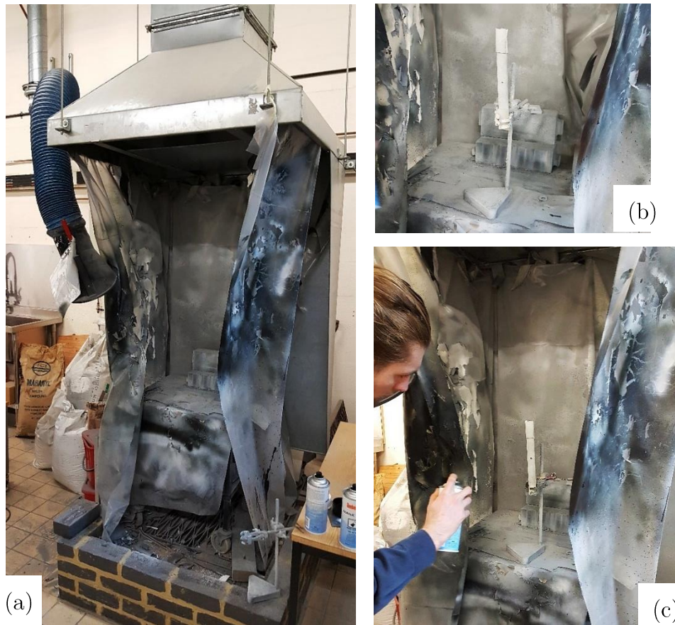
Figure 2.12: (a) Working environment with fumes cupboard, (b) specimen after the application of the white background, (c) spray painting of the black speckle pattern
