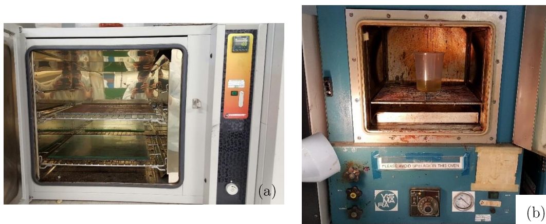
Figure 2.4: (a) glass and metal plate heated inside the oven, (b) beker with the resin at the end of the degassing process.
