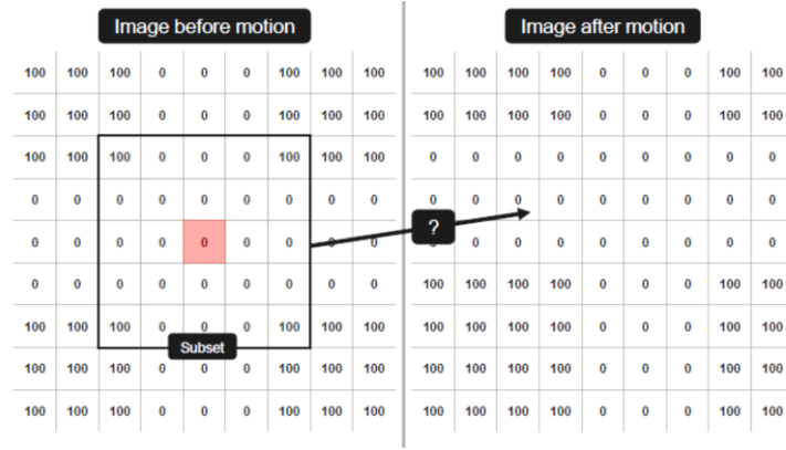
Figure 1.34: Visualization of the subset in the undeformed image and in the one after the deformation.
