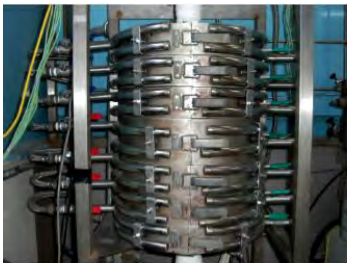
Figure 2.5. View of the seven sections of the oven surrounding the tubular reactor
