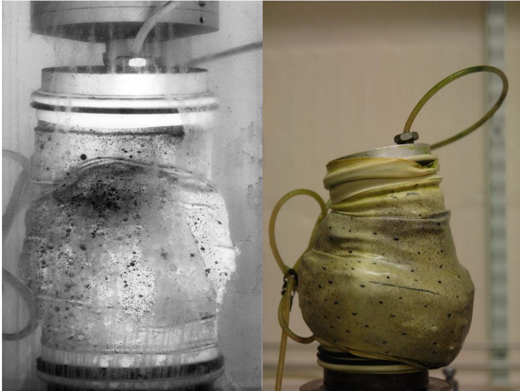
Figure 79 Specimen at the end of the test at a cell pressure of 25 kPa
