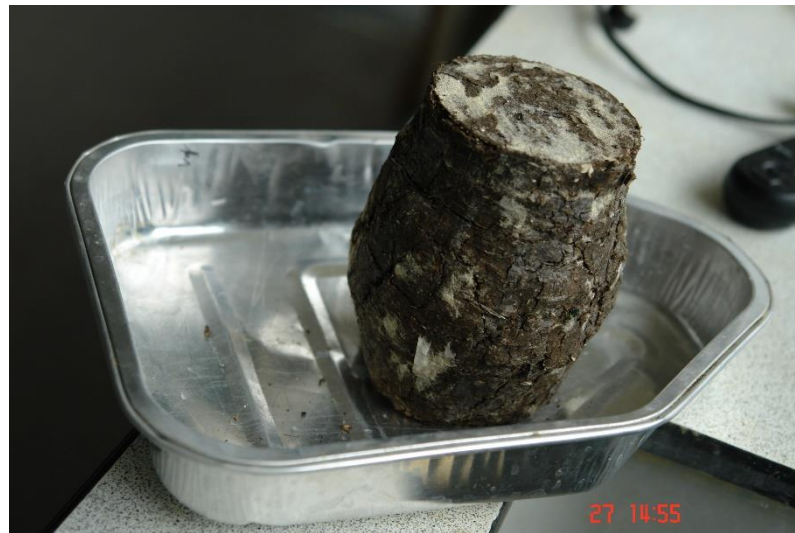
Figure 97 Dry specimen at the end of the test at a cell pressure of 200 kPa
