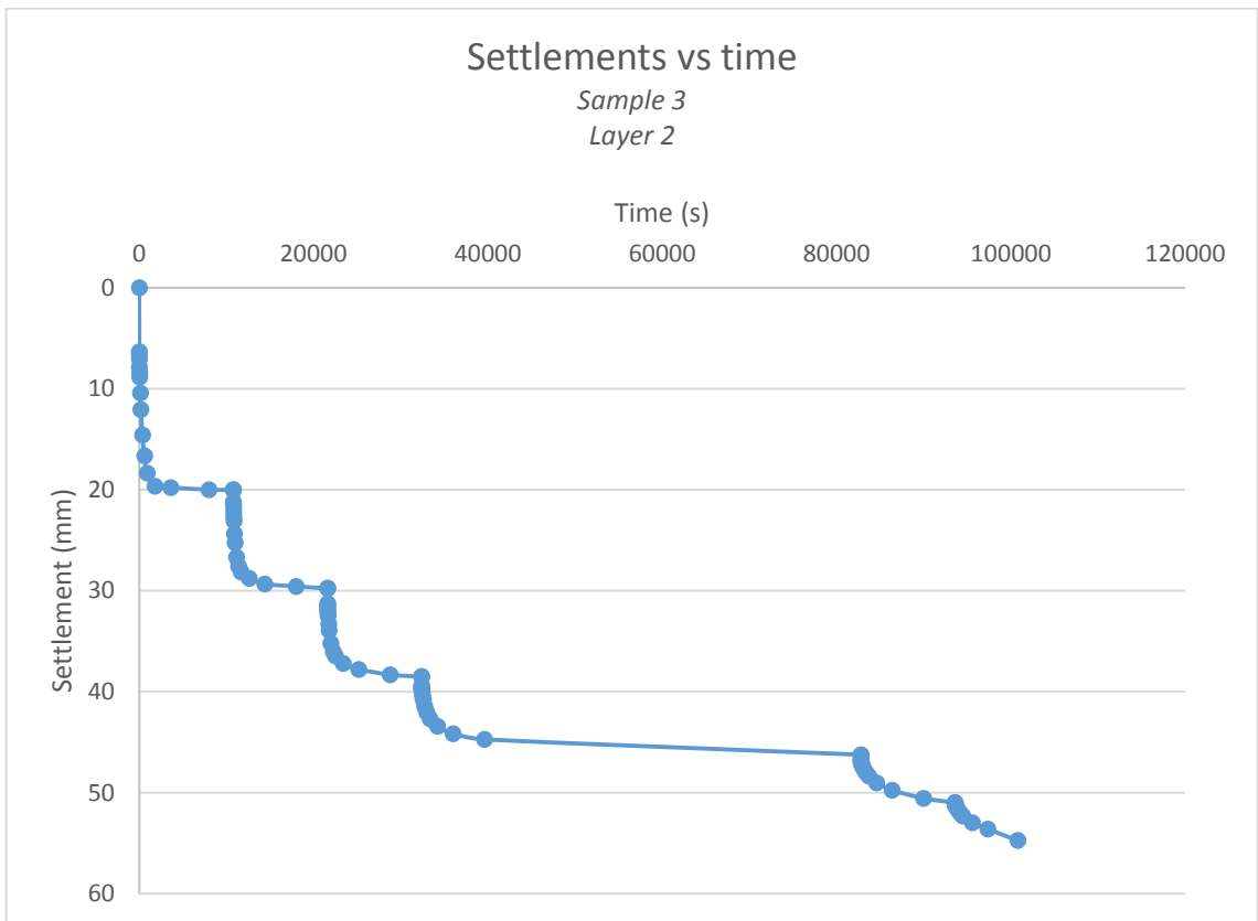
Figure 53 Oedometer test results (Sample 3; Layer 2)
