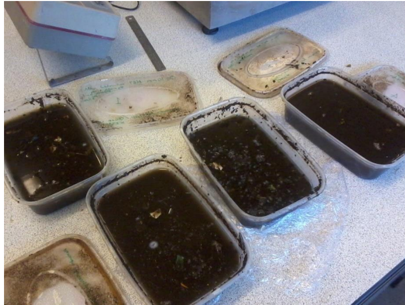
Figure 43 MBT waste mixed with acid solution three days after the sealing.
