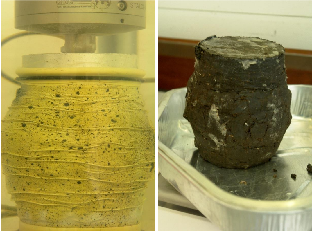
Figure 96 Specimen at the end of the test at a cell pressure of 200 kPa
