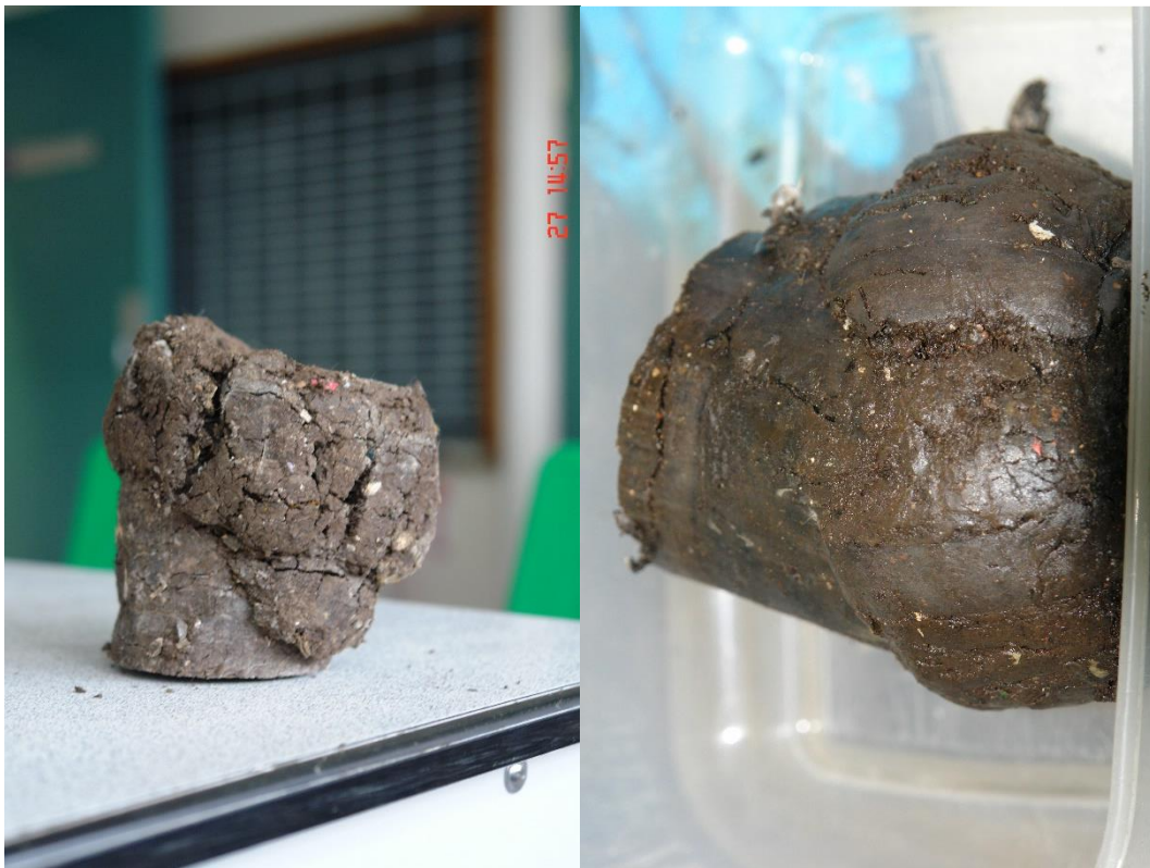
Figure 80 Dry and wet specimen after the triaxial test at a cell pressure of 25 kPa
