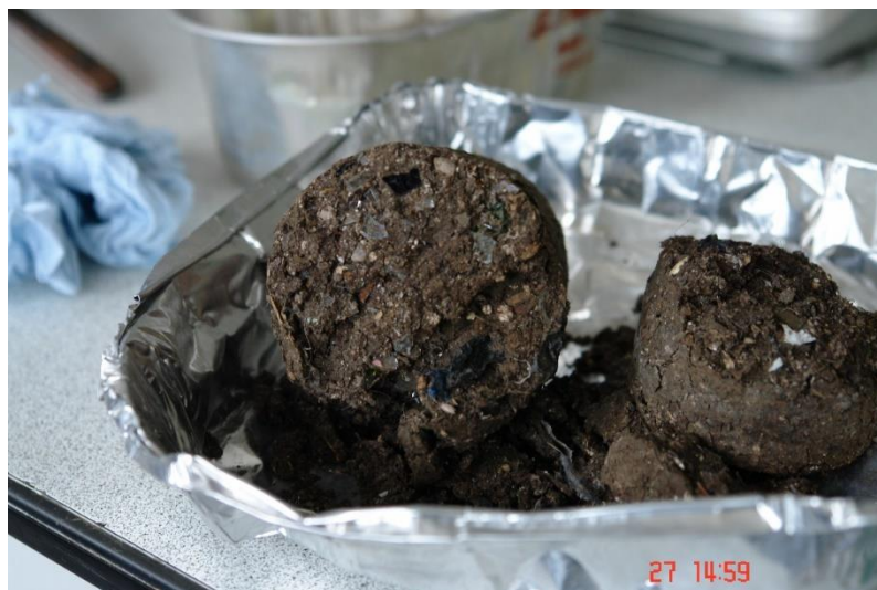
Figure 101 Inside of an MBT waste specimen.
