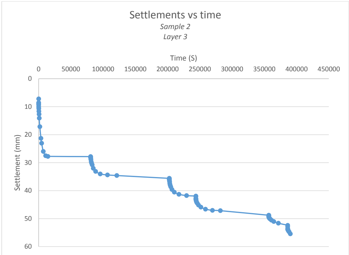
Figure 50 Oedometer test results (Sample 2; Layer 3)
