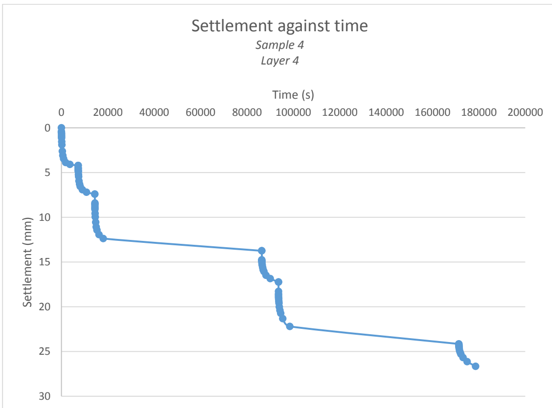
Figure 58 Oedometer test results (Sample 4; Layer 4)
