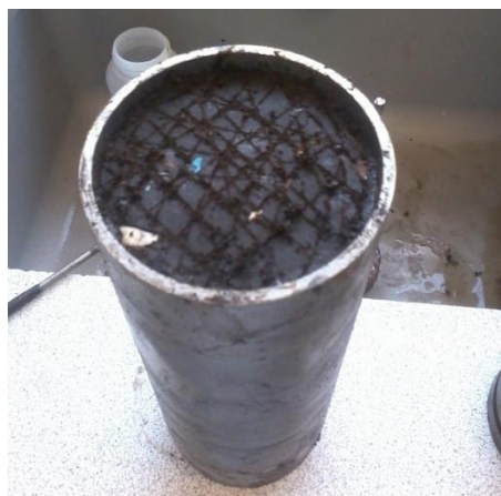
Figure 47 Scabbled surface between two consecutive layers.
