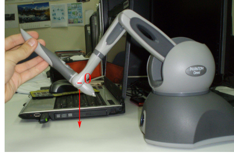
(b) To obtain a straight forward movement, the user has to bring the HIP in a negative position about y component. The arrow here is not indicating any references coordinate, it indicates just the suggested movement to perform.
