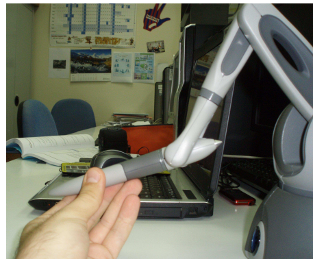
(b) Moving the tip of the stylus up, the user will be able to observe the top and, vice versa, moving the stylus down, he will see the bottom.
