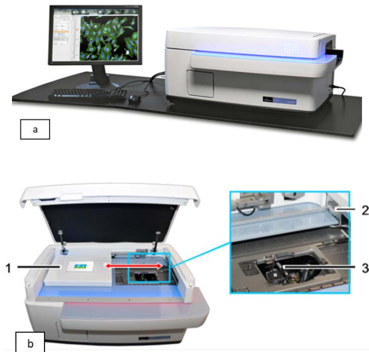
Figure 1.9 a) Overall view of Operetta® joined with a desktop computer to control and to manage the analysis; b) view of the internal components of the instrument: 1 is the live chamber, 2 is the electrical connector and 3 is the temperature sensor. (Operetta Technical Manual)
