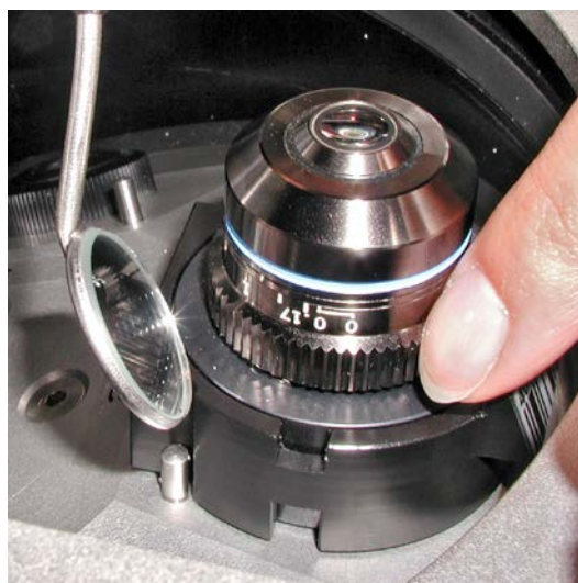
Figure 2.11 Correction collar manual settings on the objectives that include this feature (Operetta Technical Manual)
