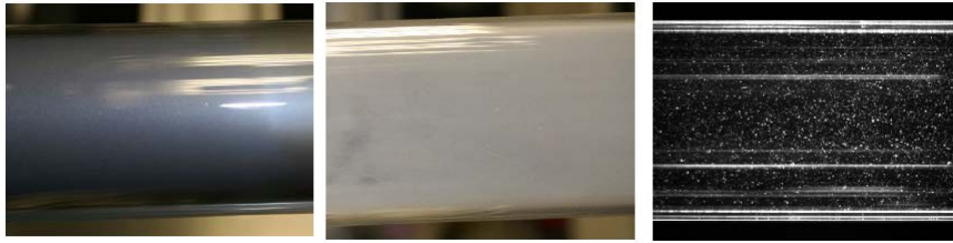
Figure 33: Material deposition [58]: Molybdenum disulphide (On the left), Boron nitride (In the center), Graphite (On the right).
