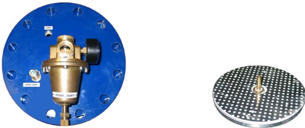
Figure 37: Seeding generator PB200 . On the right: Top view; on the left: Dispersion plate [29].
