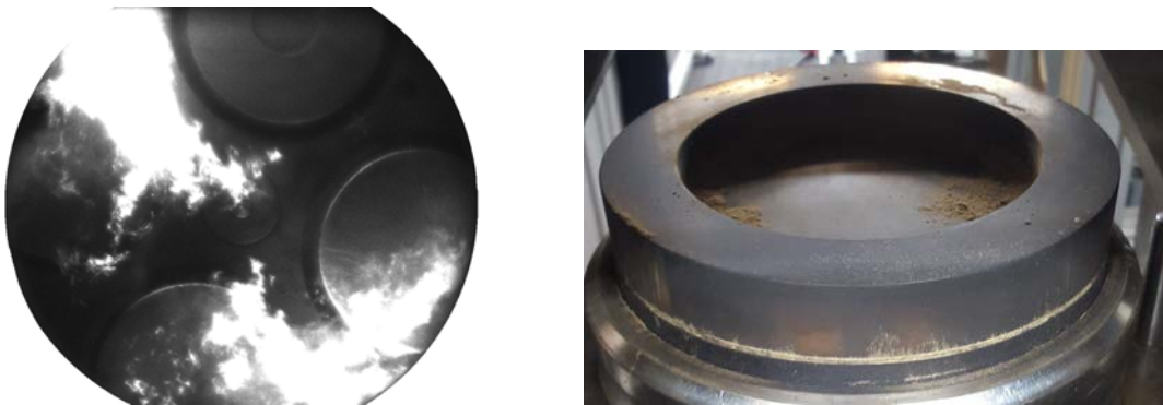
Figure 83: Lycopodium ignition and its effect in the piston.
