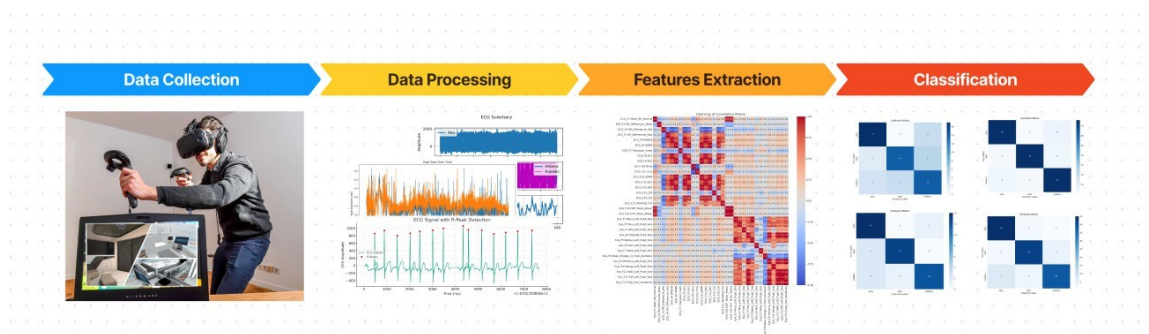
Figure 3.1: Stages of ECG and Eye Tracker Data Utilization for Cognitive Load Assessment
