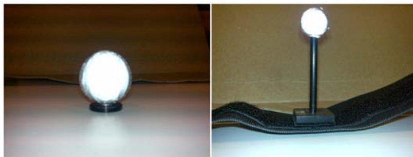
Figure 4.13: On the left normal reflecting marker, on the right a particular of a wand with the Velcro strap.
