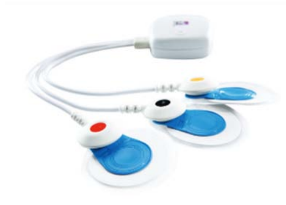
Figure 4.8: One of the sensor of the Mega WBA EMG system: the three electrodes and the wireless transmitter.
