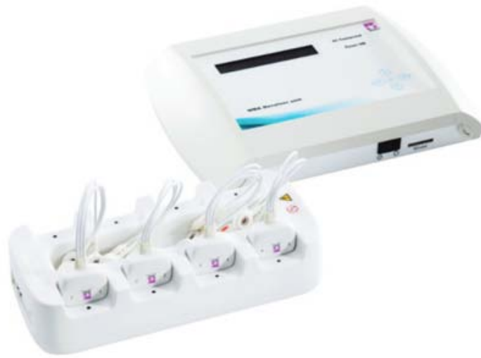
Figure 4.7: Mega WBA EMG system: above the receiver and below the sensors attached on the charging/synchronizing module.
