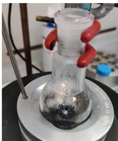
Fig. 29: Condensation of a mixture of benzylamine and water over the cold walls of the reaction flask.
