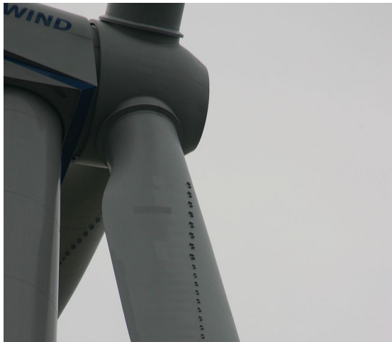
(a) Vortex generators on WT blade [10]
