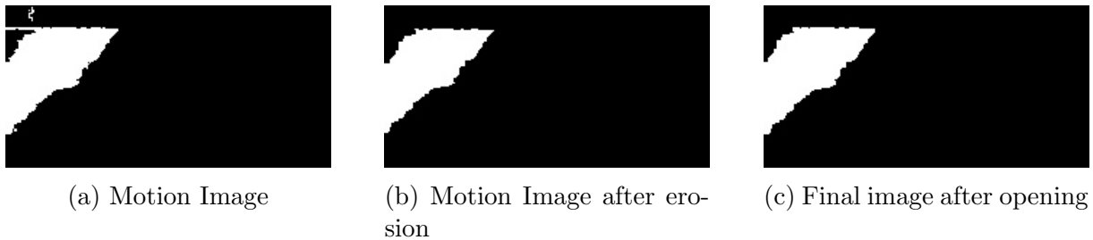
Figure 2.7: Input image and two steps of opening operation with a 3x3 kernel
