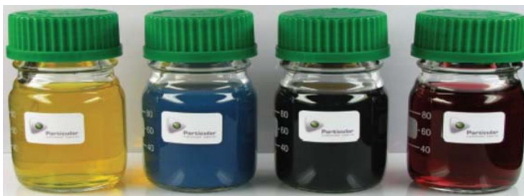
Figure 3.2 I Sol dispersion of metal nanoparticles. From left to right: silver, titanium, platinum and gold nanoparticles [49]
