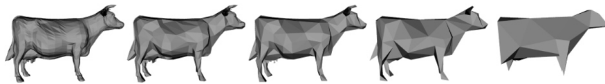
Figure 4.1: A sequence of approximations generated using Garland and Heckbert’s algorithm [33]. The original model on the left has 5,804 faces. The approximations to the right have 994, 532, 248, and 64 faces respectively.
