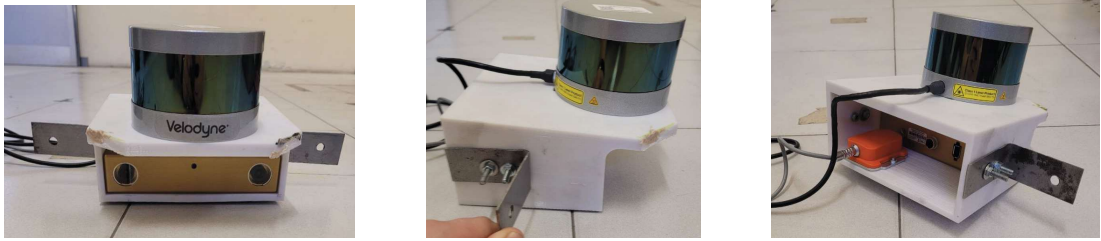
Figure 7.5: Front, side, and back view of the developed sensors support.
