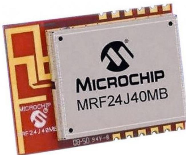
Fig. 17 Modulo radio MRF24J40MB-I/RM
