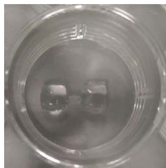
Figure 3.19. Second structure designed for cellular tests with SK-N-AS cells, bioprinted with rectilinear pattern infill in a multiwell plate.
