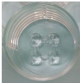
Figure 3.17. First structure designed for cellular tests with SK-N-AS cells, bioprinted with circular pattern infill in a multiwell plate.
