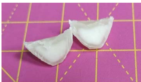
Figure 3.1. GelMA obtained with Method A, purified with ethanol, and vacuum-dried; clearly not dried in the inner part.
