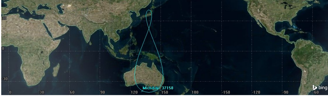
Figure 2.3: Ground track of QZS-1 created with the System Tool Kit (STK) of Analytical Graphics Inc. AGI. The day selected for the plot is January, 15 2017.
